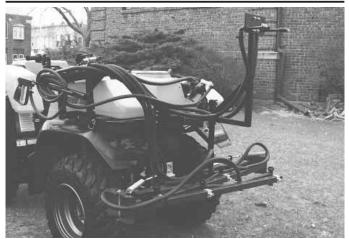
Kit includes 25-gal. tank, bracket, and two boomless nozzles that mount on ATV. (Note: 12-ft. boom on ATV shown above was used by a chemical company for test plot work.) 30-ft. spray pattern. The angle of the nozzles 30 ft. to its effective length."
