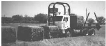
"Haying Mantis" mounts on any cab-over semi-truck and automatically brings bales up and over the cab. Flatbed lifts up 90 degrees to stack bales on ground.
