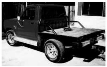
Brittin cut off the back part of a wrecked Ford Bronco, attached part of a Ford Ranger pickup cab, and added his own remote-controlled hydraulic tilt bed.
