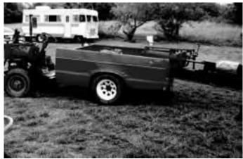
Splitter mounts on cut-off pickup bed pulled by a 40 hp Wisconsin engine.
